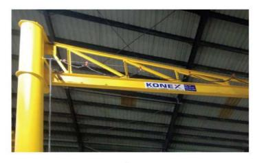
shops, loading & unloading purpose etc. Dedicated JIB cranes for a single workstation allow efficient material handling by reducing waiting time for an overhead crane. JIB cranes are mainly available manual-swing operated with Wire Rope Electric hoists, with/without pillar and capacities up to 3 Ton
