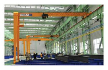
indoors and outdoors. Semi Gantry Cranes are available in capacities up to 20 Ton
