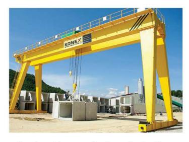
production and manufacturing facilities as well as in outdoor applications. Gantry Cranes are available in capacities up to 30 Ton
