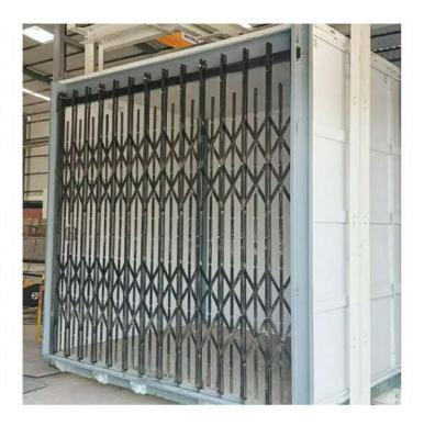
The construction of cage will roll steel section and sides will be covered with Bump Sheets. Top of cage will be covered with M S Sheets & bottom will be made from chequered plate. Collapsible doors are provided in cage as per entry & exit requirement at site
