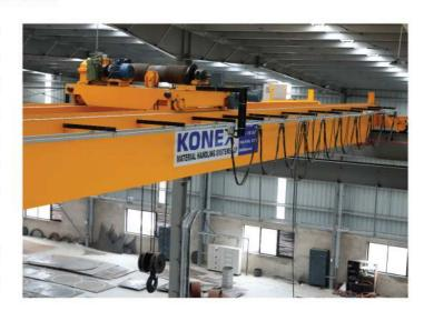
Double Trolleys / Auxiliary hoisting mechanism can be provided in Double Girder EOT Cranes.
